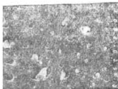
Fig. 8 Electron micrograph of PAC/AS film coagulated in water
